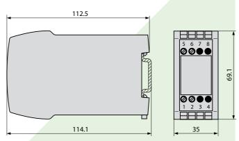
Fig. 3. SINEAX U 543 in housing  $\it P8/35$  clipped onto a top-hat rail (35 ×15 mm or 35×7.5 mm, acc. to EN 50 022).
