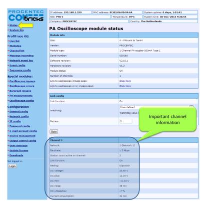
Fig. 84 - PA Oscilloscope module status
