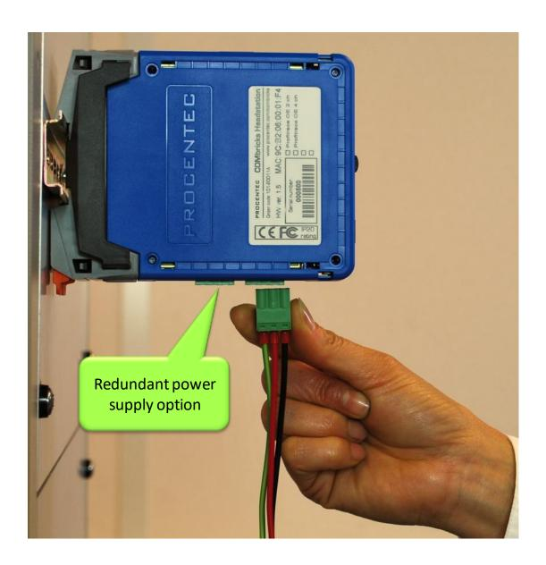
Fig. 23 - Head Station power supply
