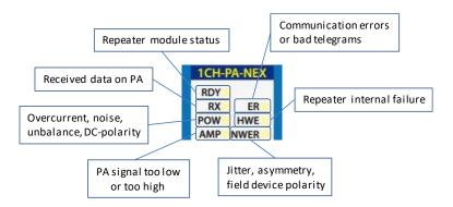
Fig. 82 - Overview of LEDs
