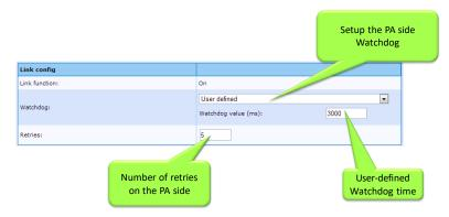
Fig. 89 - Configuration of bus parameters on PA
