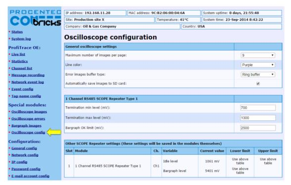
Fig. 48 - Oscilloscope configuration
