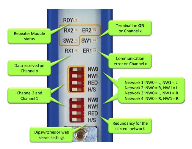
Fig. 24 - Dipswitches and LEDs of the repeaters
