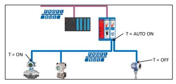
Fig. 91 - PA segment with a stub line
