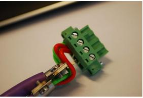
Fig. 26 - Use the Dual Ground Clip to connect two PROFIBUS cables in one screw terminal
