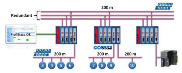
Fig. 59 - Application with 3 redundant segments
