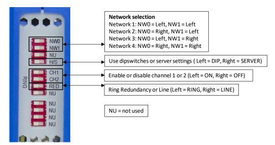
In all ring redundancy modes, the Ring dipswitches must be switched to the LEFT position.
