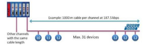
Fig. 57 - PROFIBUS DP cable lengths
