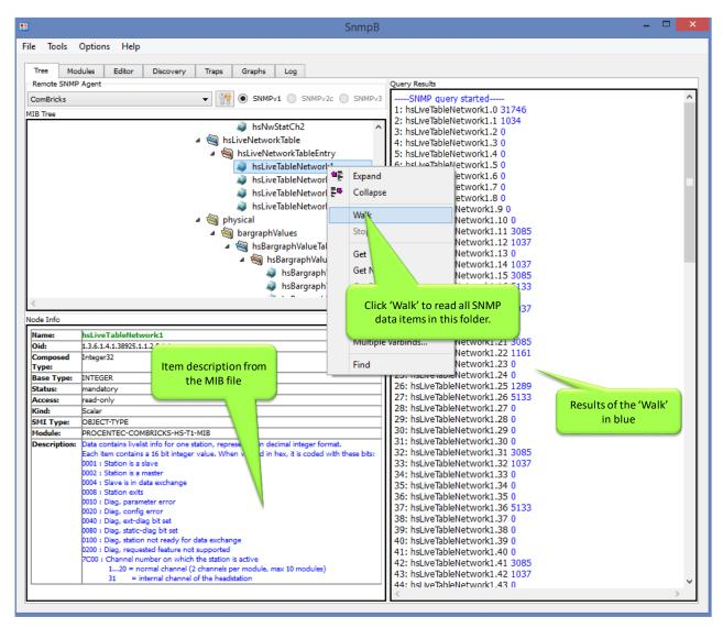
Fig. 114 - Example of reading SNMP data
