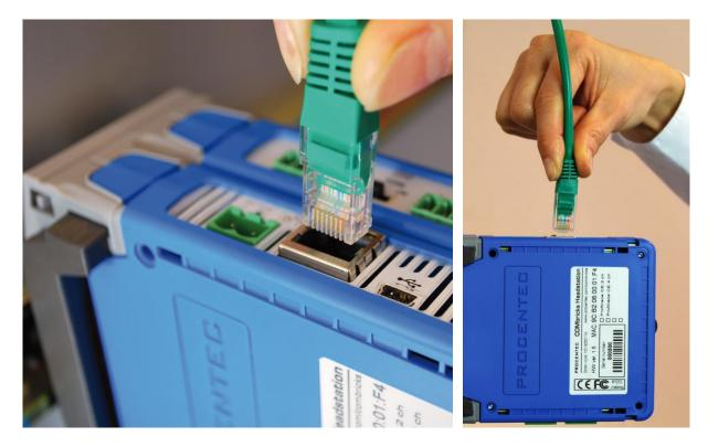
Fig. 22 - Wiring Ethernet
