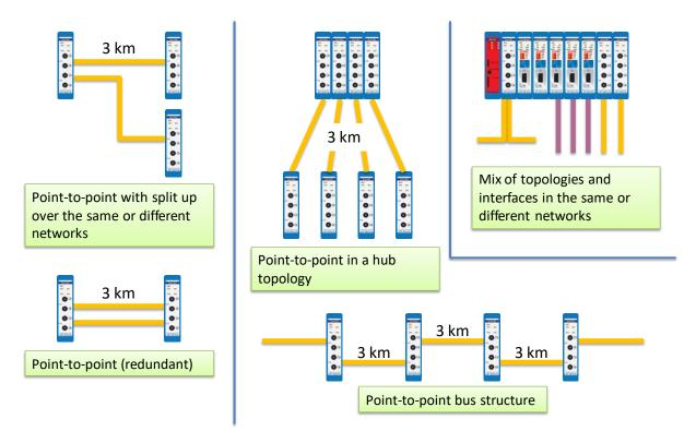
Fig. 61 - Fiber optic topologies
