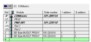
Fig. 102 - Configuration for PROFINET network 1
