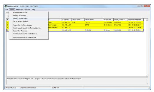
Fig. 94 - Assigning a new device name
