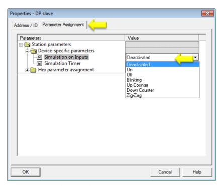
Fig. 73 - Input simulation window
