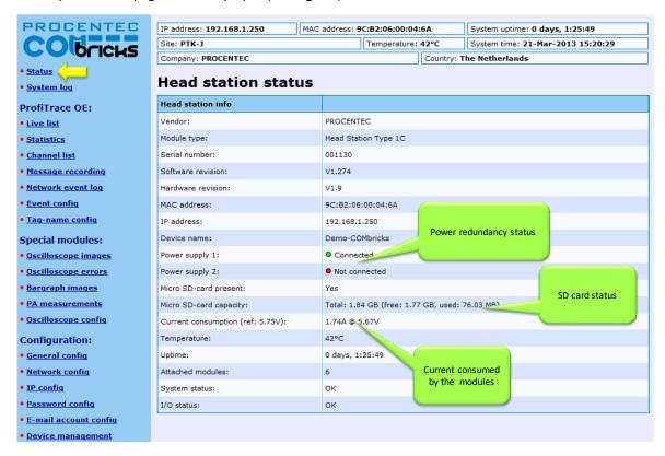
Fig. 28 - Example of a module status
