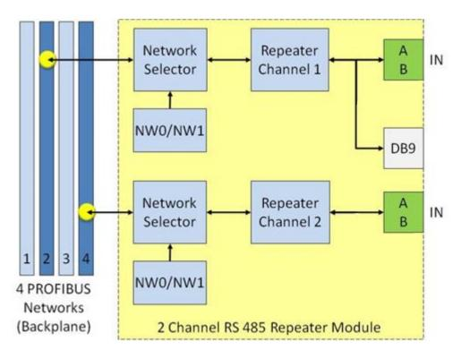
Fig. 54 - Multiple channels per module
