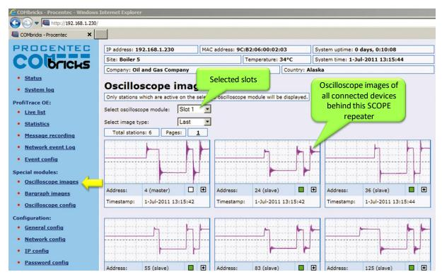
Fig. 47 - Oscilloscope images from all devices
