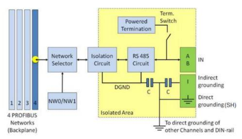
Fig. 55 - Channel structure of the repeater modules
