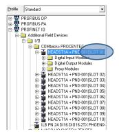
Fig. 97 - Select the device with correct slot number
