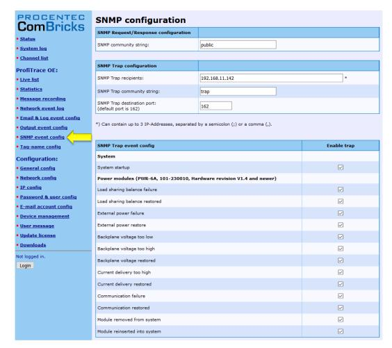
Fig. 45 - SNMP trap setup page
