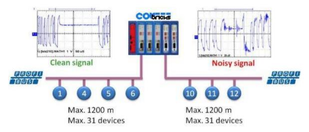
Fig. 56 - ComBricks as EMC barrier
