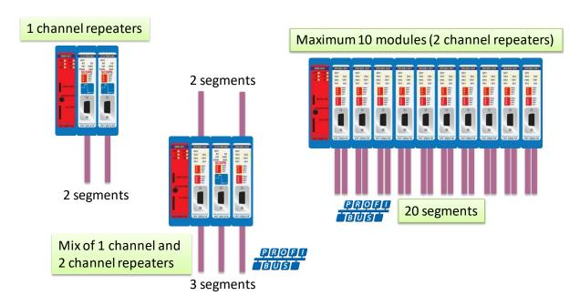
Fig. 2 - Repeater configuration examples
