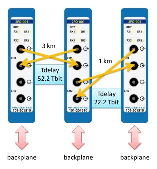
Fig. 62 - Fiber optic delay time
