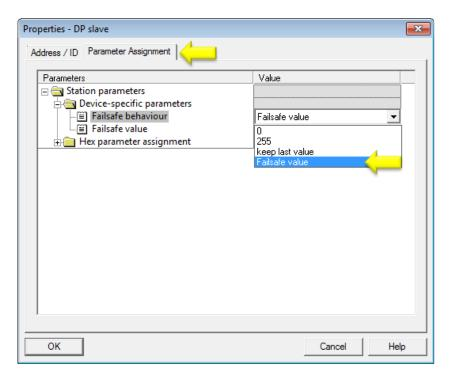
Fig. 72 - Parameter assignment window
