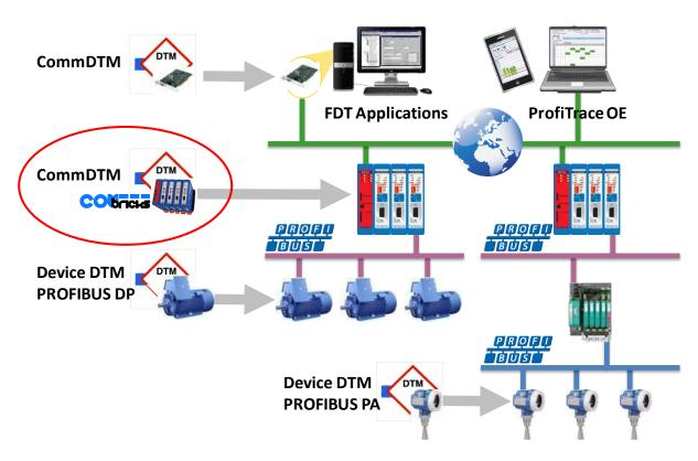
Fig. 11 - CommDTM structure
