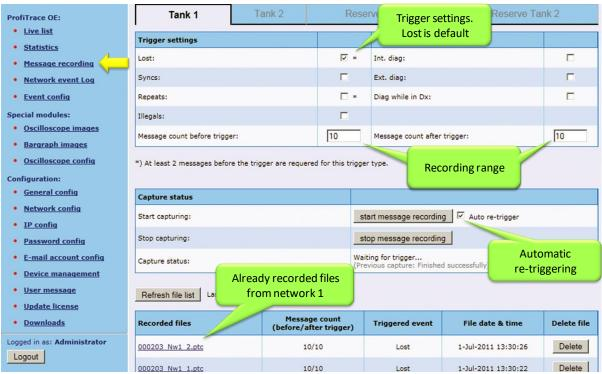
Fig. 43 - Setup recording trigger
