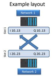
Slot 1 belongs to Network 1. Slot 2 is connected to Network 2. These networks can now be coupled via the configuration tools of each master. For example, if you want to transfer 1 byte, the setup for the configuration tool of network 1 will look as follows:
