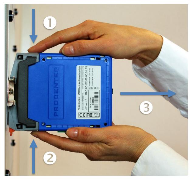
Fig. 21 - Removing modules
