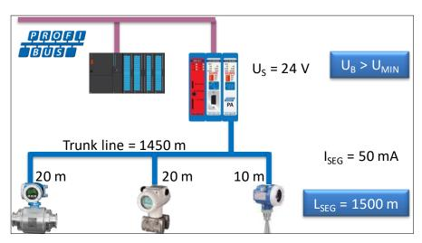
Fig. 93 - Example of voltage calculation at the end of the cable
