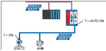
Fig. 90 – PA segment using one connector
