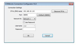
Next, select this location again and click 'Setup'. Enter the correct IP address of the ComBricks Head Station, and choose the port and network you wish to connect to. Depending on the password settings in the ComBricks, you might also have to fill in a username and password. Then click 'Ok'.
