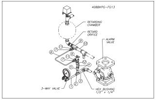
Figure 13—Closed Retard Drain. UL Listed.
