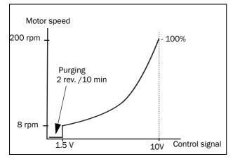
Fig. 2 Relation between control signal and motor speed -Normal conditions
