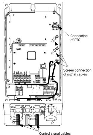
Fig. 12 Connecting the control signals and PTC
