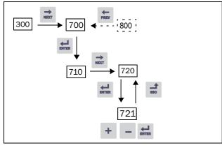
Fig. 15 Example of menu navigation when checking VSD status
