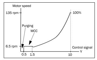
Fig. 3 Relation between control signal and motor speed when using special MCC parameters, see further in chapter 7.2.1 page 27.
