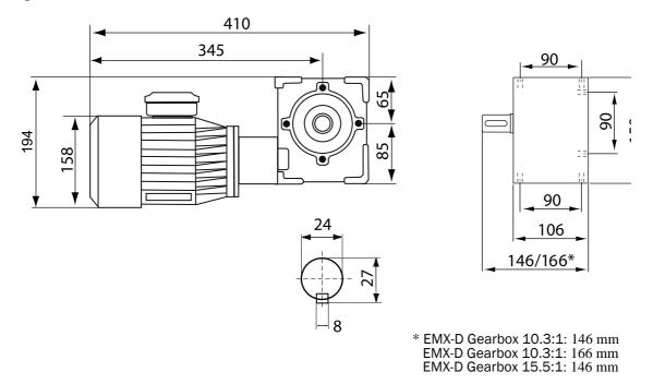
Fig. 37 Dimensions, motor and gearbox (mm)
