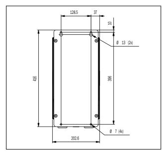
Fig. 5 Control unit mounting scheme
