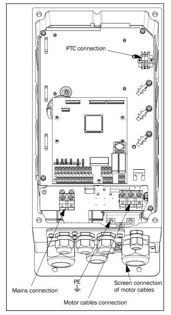
Fig. 7 Mains, motor and PTC connections to Control unit.
