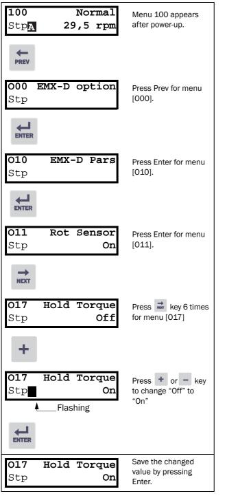
Fig. 26 Programming example 3, Turn on the Hold torque.
