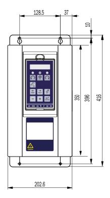
Fig. 36 Dimensions, control unit
