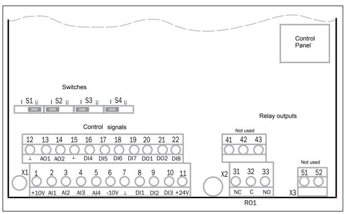
Fig. 10 Control board layout
