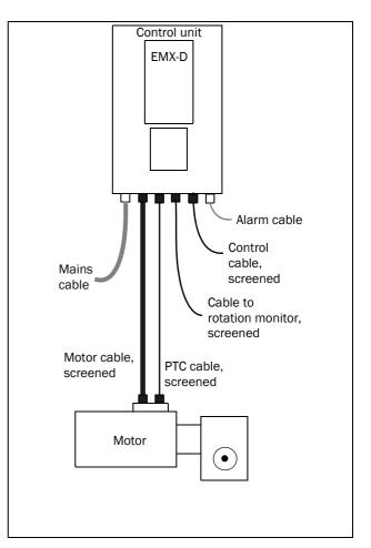
Fig. 9 EMC-adapted installation of EMX-D
