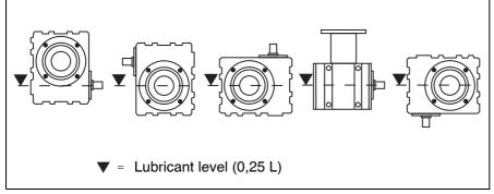
Fig. 1 Recommended oil level in the gearbox depending on shaft position.
