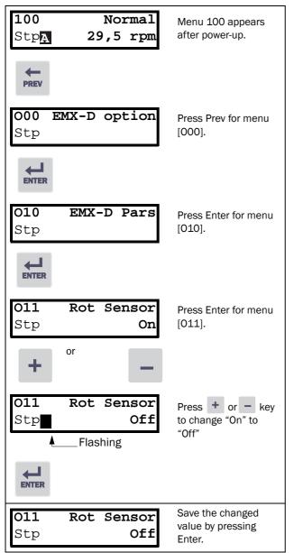
Fig. 24 Programming example 1 Turn off Rotation sensor
