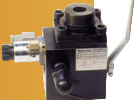
They are designed to incorporate in a single compact block the variety of functions necessary for the correct operation of an hydraulic system fitted with accumulators. This includes manual and/or electric drain, isolation, flow control and pressure relief. Channel cross section : 10 mm (DI 10 block), 16 mm (DI 16 block), 20 mm (DI 20 block), 24 mm (DI 24 block), 32 mm (DI 32 block).
