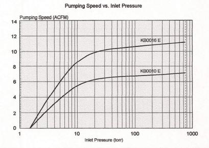
Technical Data KB 0010 E KB 0016 E Nominal pumping speed ACFM Ultimate pressure Torr Motor power kW (Hp) Nominal rotational speed RPM Sound level rating\* dBA Weight (approx.) Lbs. Oil capacity (approx.) Qts.
