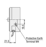
Detail Drawing of Protective Earth Terminal
