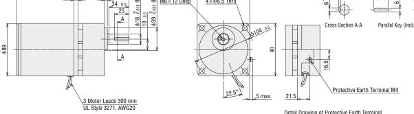
Detail Drawing of Protective Earth Terminal
