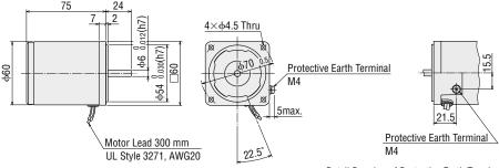
Detail Drawing of Protective Earth Terminal
