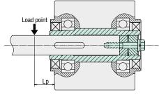
Lp [mm]: Distance from flange-installation surface to radial load point
