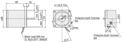
Detail Drawing of Protective Earth Terminal
