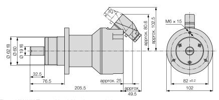
Fig. 6. KINAX WT 707 with additional gear and plug connector.
