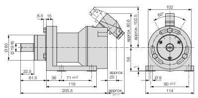
Fig. 10. KINAX WT 707 with additional gear, plug connector and foot.
