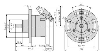
Fig 12. KINAX WT 707 with plug connector and flange.
