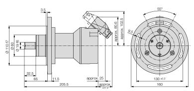
Fig. 14. KINAX WT 707 with additional gear, plug connector and flange.
