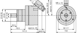
Fig. 4. KINAX WT 707 with plug connector.
