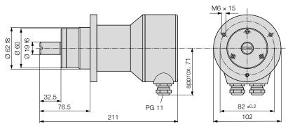
Fig. 7. KINAX WT 707 with additional gear, screw terminals and cable glands.
