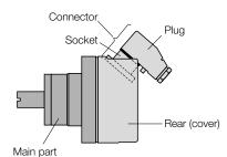
Fig. 1. Cable outlets towards the back
