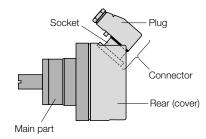
Fig. 2. Cable outlets towards the front
