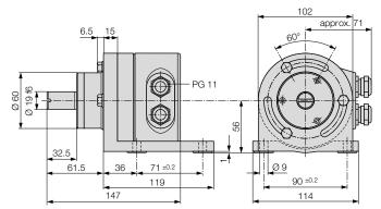
Fig. 8. KINAX WT 707 with plug connector and foot.
