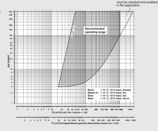
$$f = \sqrt{\frac{\text{Air density}}{\text{Density of the gas used}}}$$
