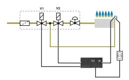
Atmospheric burner with ignition gas output.
