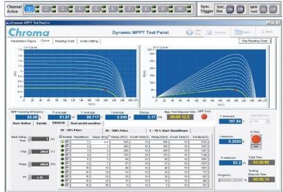
Solar Array Simulation Softpanel
