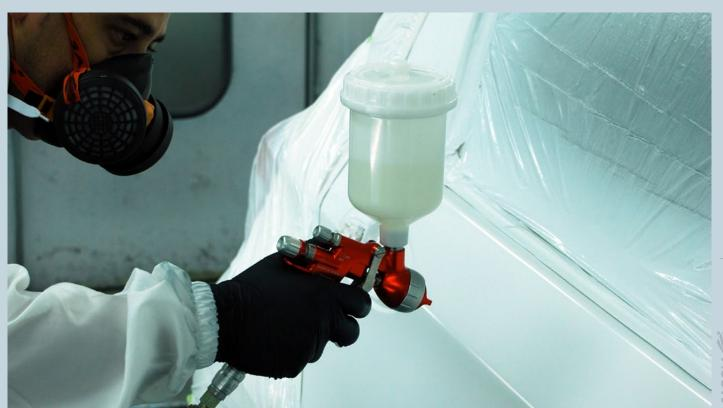
**The aircap model** is vital to achieve the desired results. The type of product we are going to apply and the application system we are going to use must both be taken into account when selecting an aircap. We will obtain the desired spray by correctly combining the aircap with the correct nozzle and needle kit, and a proper air supply.
