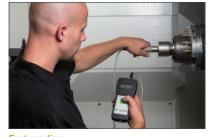
A precision force sensing bar with expansion measuring strips performs the measurement.
