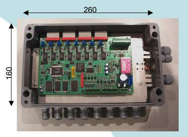
Housing height: 90mm Fixing screw spacing: 240 x 110 mm, fastening material is supplied.
