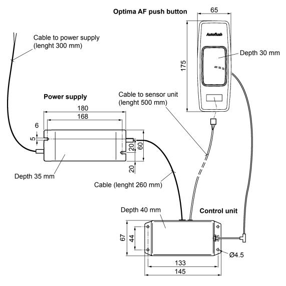
Materials Control unit; bellows: rubber, cover and bottom of control box: ABS
