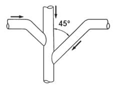
if a branch pipe is connected to the main line from above. (For example, when connecting branch pipe to a horizontal main line), the branch pipe must be connected with a smooth bend to the upper side of the main line with a 45° angle.
