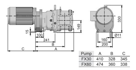
Materials Pump housing: Cast iron GG25, mat. no. 0.6025
