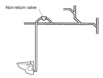
In case the riser height exceeds 3 m the vacuum connection should be placed at the top of the riser.
