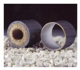
After several years of intensive use, the diameter of the vacuum pipes can shrink because of the scale and concentrated urine that precipitate. It exists cleaning products made of concentrated acidic, but they may be dangerous for the operator, to the treatment plant, to the joints and to the environment.
