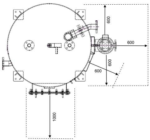
(Min. maintenance distances in mm, top view)
