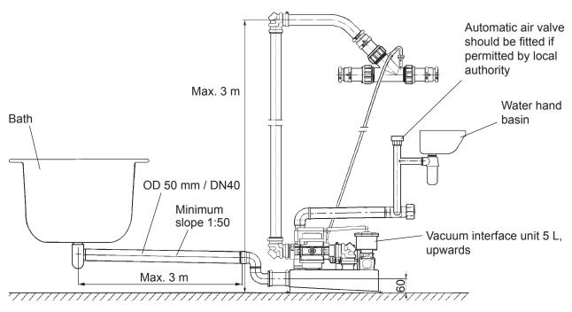
! NOTE: The maximum flow to the vacuum interface unit from all appliencies must not exceed:
