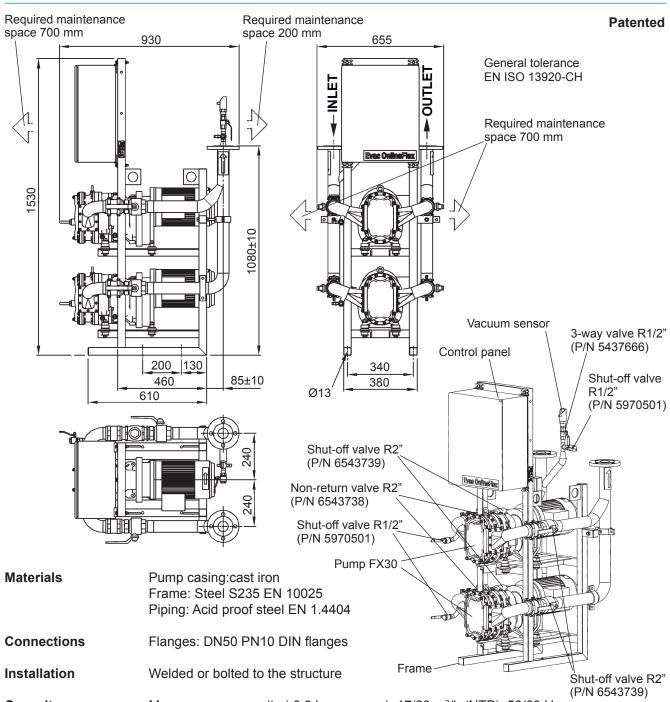
Capacity Max. vacuum capacity (-0.3 bar vacuum): 17/20 m³/h (NTP), 50/60 Hz
