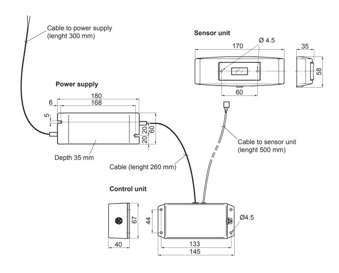
Materials Control unit; bellows: rubber, cover and bottom of control box: ABS
