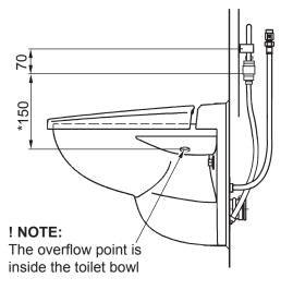
\* The vacuum breaker air inlet must be located at minimum of 150 mm (6") above overflow point of the toilet.
