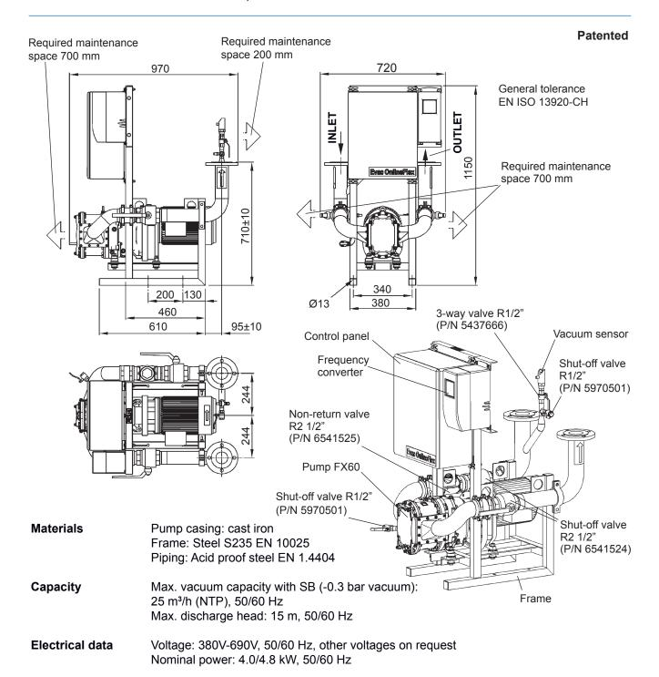
**Connections** Flanges: DN65 PN10 DIN flanges
