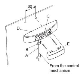
Installing the push button on the wall, floor models with the optional push button kit.
