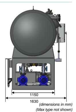
Total vacuum capacity m<sup>3</sup>/h **Power KW** Dry weight Kg **Type** 30 HQE 140 R2 13.5 1520 252 **30 HQE 140 R2 MAX** 15 1570 252 30 HQE 160 R2 MAX 14 1610 288 **30 HQE 200 R2 MAX** 16.4 1630 360 **30 HQE 250 R2 MAX** <del>18</del> <del>1640</del> <del>450</del> **30 HQE 300 R2 MAX** 20 1640 540
