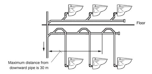
Riser pipe with lift 3 ... 5 m lift is allowed only immediately after a toilet and back flow must be prevented by a transport pocket and non-return valve.
