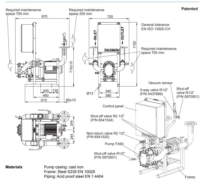
Capacity Max. vacuum capacity (-0.3 bar vacuum): 17/20 m³/h (NTP), 50/60 Hz
