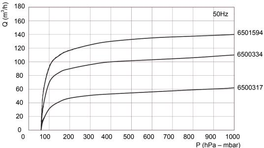
The displacement curves are valid for air at 20 °C. Tolerance: ± 10%
