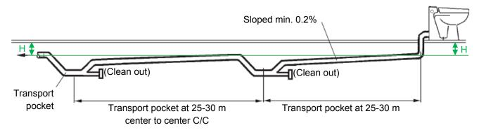
**Allowable pipe profile:** Pocket at every lift, horizontal pipes, the sum of risers (H1+ H2 + H3+...) should always remain below 3 m.
