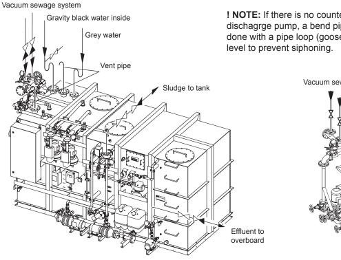
! NOTE: If there is no counter pressure for the dischagrge pump, a bend piping arrangement must be done with a pipe loop (goose neck) over tank's water
