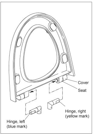
2. Push the hinges into the hole of the seat and the cover.
