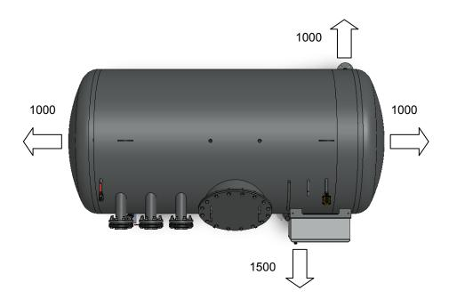
(Min. maintenance distances requirement in mm)
