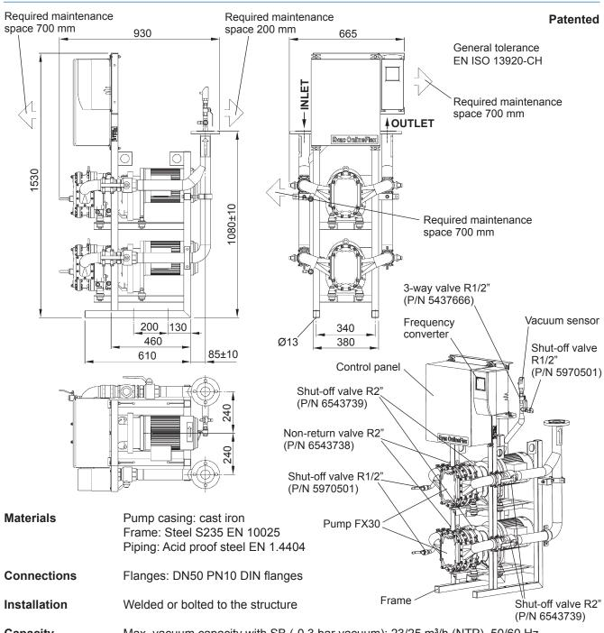
Capacity Max. vacuum capacity with SB (-0.3 bar vacuum): 23/25 m³/h (NTP), 50/60 Hz
