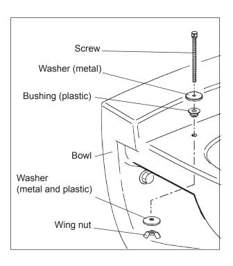
1. Install the parts of the installation kit. Note installation order.
