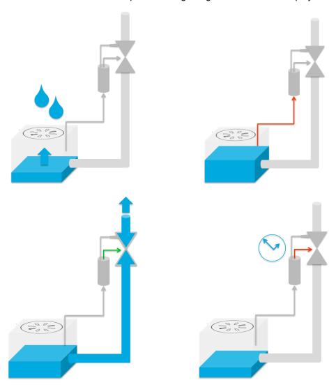
Sequences of an Evac floor drain operation
