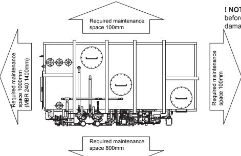
! NOTE: Fill the tank with water before welding to avoid painting damages during welding.
