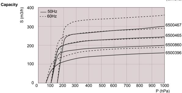
The displacement curves are valid for air at 20 °C. Tolerance: ± 10%
