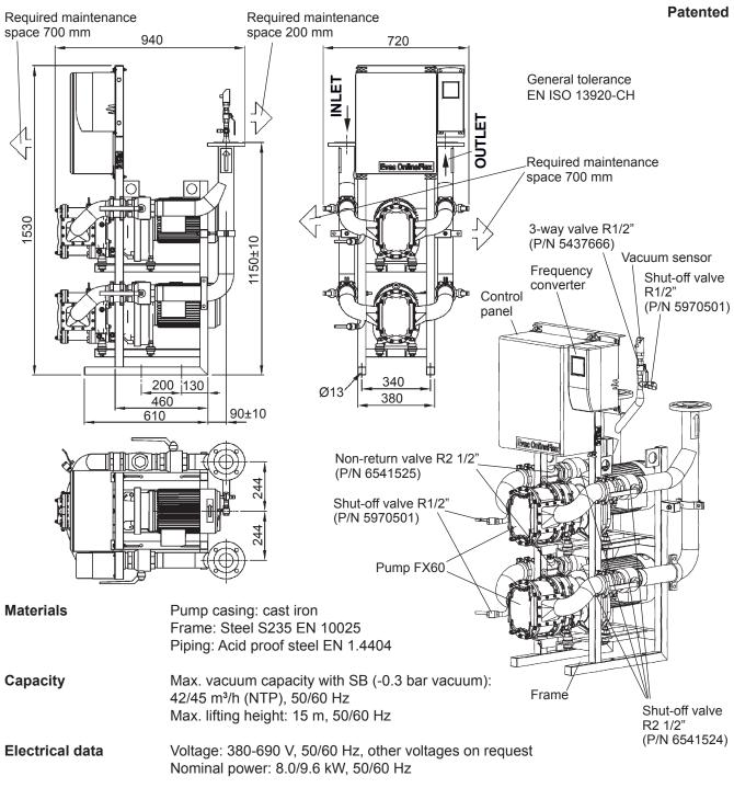
Connections Flanges: DN65 PN10 DIN flanges
