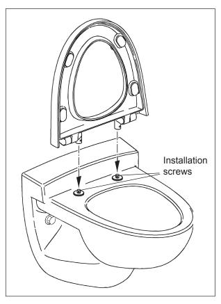
3. Install the seat and the cover with the hinges on the installation screws on the bowl.
