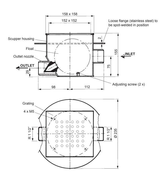
! NOTE: Incoming gravity line must be ventilated above the highest sanitary fixture.
