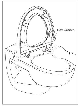
4. Tighten the retaining screws with a hex wrench. (The installation kit includes two hex wrenches.)
