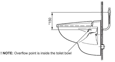
\* The vacuum breaker air inlet must be located at a minimum of 150 mm (6") above the overflow point of the toilet.
