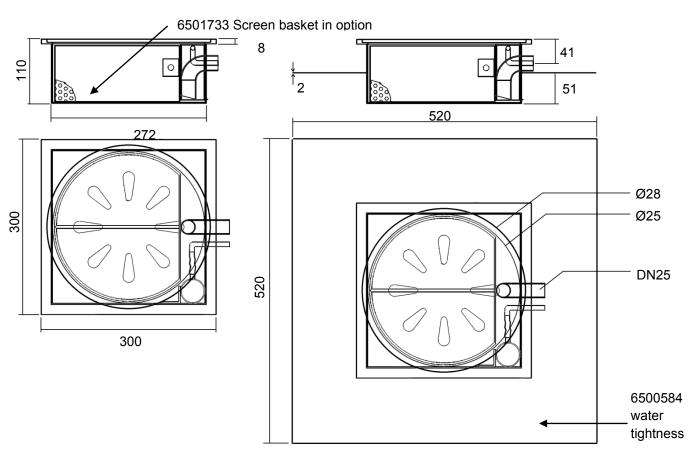
Configuration for installation without water tightness
