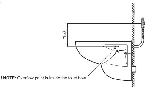
\* The vacuum breaker air inlet must be located at a minimum of 150 mm (6") above the overflow point of the toilet.
