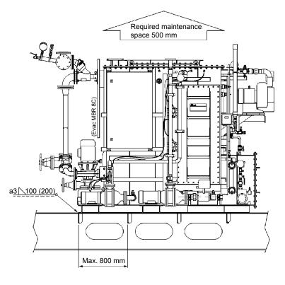
! **NOTE**: The installation frame/deck must be flat and level.
