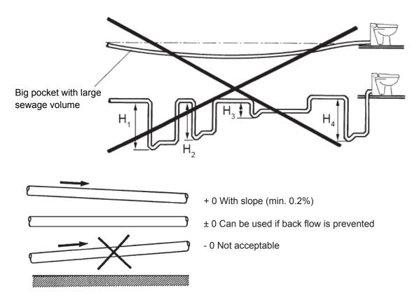
Horizontal pipes shall run either downwards in the direction of the flow or horizontally, never with a steady upward gradient.
