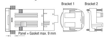
The instrument electronics can be extracted from the front side of the housing: prior to extract the instrument from the housing, disconnect the power supply.
