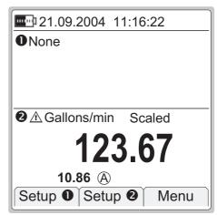
When Scaling display is active, the entered unit (or the text "scaled unit" if the unit was not entered) is displayed after the warning triangle and the text "Scaled" is shown above the Scaled value.
