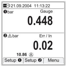
When Error In Input Units display is active, the warning triangle is shown together with the input unit and the text "**Err** / **In**" is shown above the Error value.
