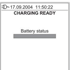
The charging time depends on calibrator's current consumption (backlight, mA sourcing etc.). With no extra load, the charging time is approx. 5 hours.
