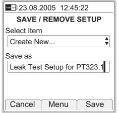
In the leftmost picture above, three User Setups are already saved. Selecting Save / Remove Setup option opens the **SAVE / REMOVE SETUP** window allowing you to save the current settings for window **1** and window **2** (see rightmost picture).
