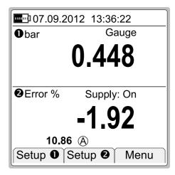
When Error Percentage display is active, the words "**Error** %" is displayed after the warning triangle.
