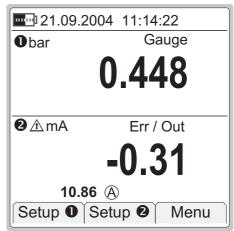
When Error In Output Units display is active, the warning triangle is shown together with the input unit and the text "**Err / Out**" is shown above the Error value.
