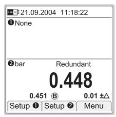
When Redundant measurement is active, text "**Redundant**" is shown above the main measurement value.
