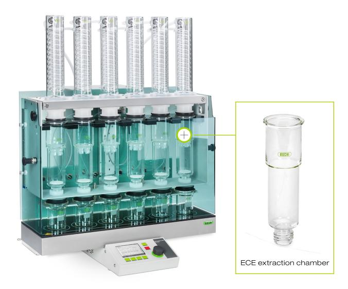
Extraction Unit E-816 ECE 6 samples in one run
