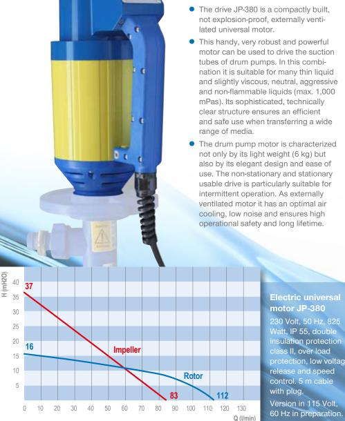
JP-380, 230 VAC, JP-PP(HC)41-1,000, test media water 20°C, pressure pipe 1", oval gear meter, measured values: ± 5%
