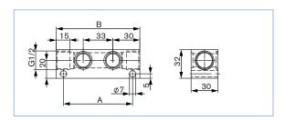
Double channels manifolds (for pressure and exhaust port) with mounting screws M5x60 DIN 912 and O-rings 11x2.5
