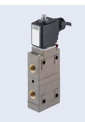
The approval Ex m is achieved by the mounting of an approved push-over coil. The cable connection and the cable are non-detachable and sealed together with the valve. The valves can be used individually or in blocks.
