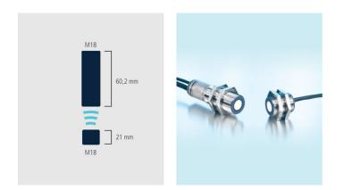
The standard: receiver and all the evaluation electronics are housed in an M18 threaded sleeve, which is only 60.2 mm long. The transmitter is housed in an M18x21 mm threaded sleeve and a 2-pin plug connects it to the receiver.
