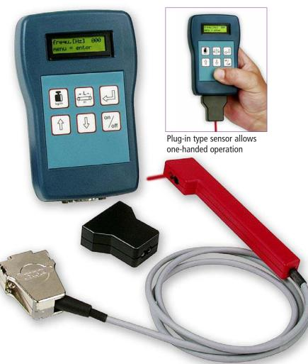
The BTM-400PLUS's LED-optical sensor is unaffected by ambient noise, offering improved performance versus competitive, acoustic sensor-based designs
