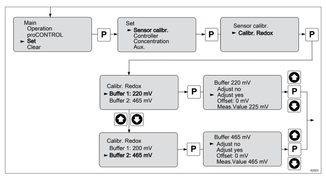
Fig. 28: Calibrating the sensor for Redox
