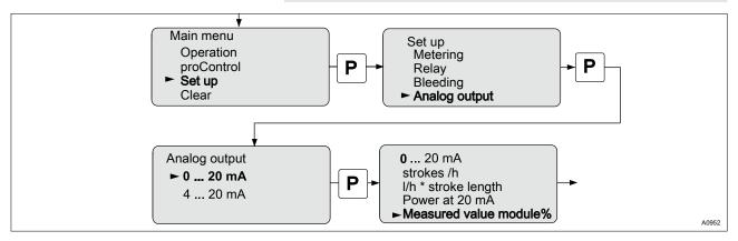
Fig. 24: Current output activation menu
