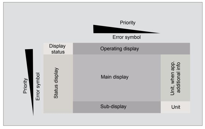
Fig. 29: Overview of the operating indicator of the delta® solenoid metering pump
