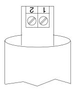
Fig. 6: Connection of the sensor or measuring transducer; 2-conductor external cable
