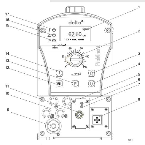
Fig. 11: Operating elements of the delta® solenoid metering pump
