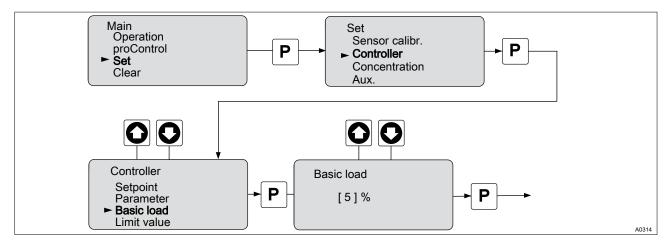
Fig. 17: Setting the basic load
