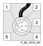
Fig. 8: Assignment on cable / 2-conductor external cable
