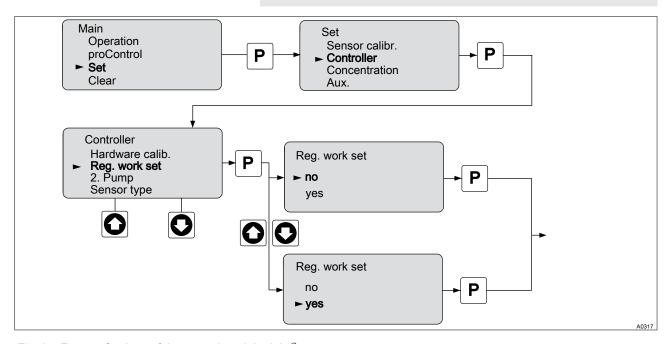
Fig. 21: Factory Settings of the control module delta®
