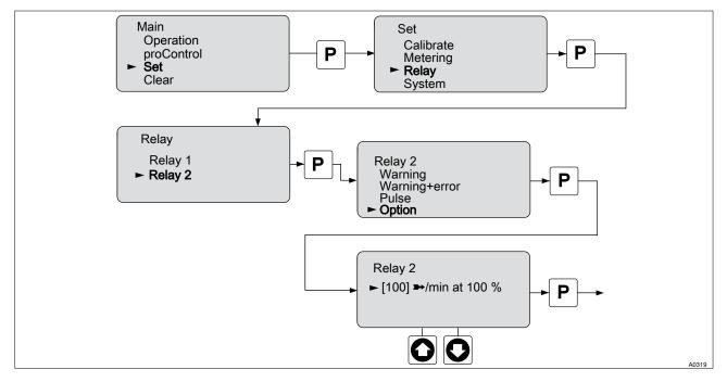
Fig. 23: Menu for adjusting the controller pulse of the second pump
