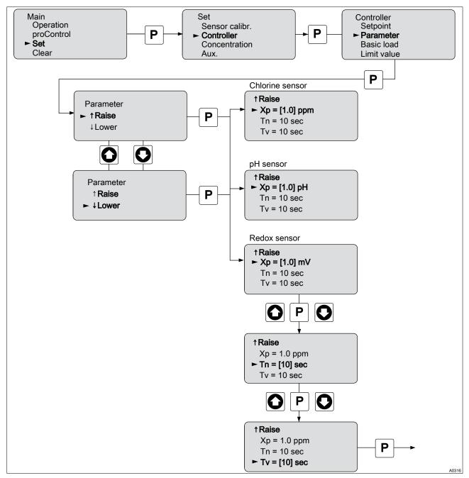
Fig. 20: Setting the control module delta®
