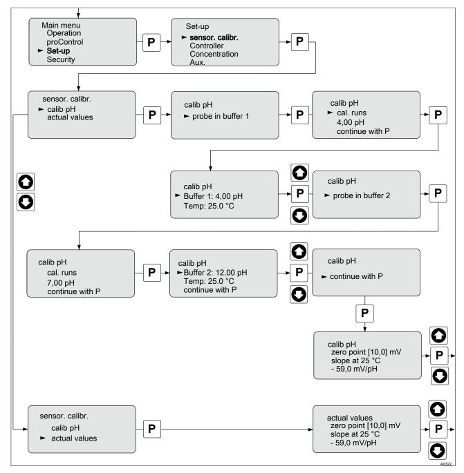
Fig. 27: Sensor pH calibration
