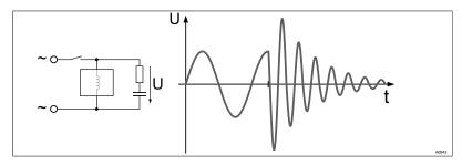
Fig. 9: Switching-off process shown on the oscillogram.
