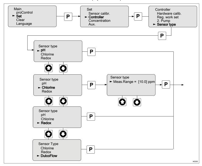
Fig. 15: Selection of the Measured Variable and Measuring Range
