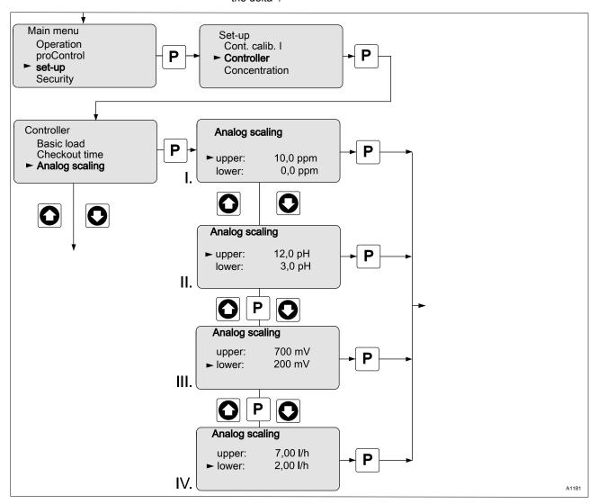
Fig. 25: Scaling the Output Value of the Analog Value
