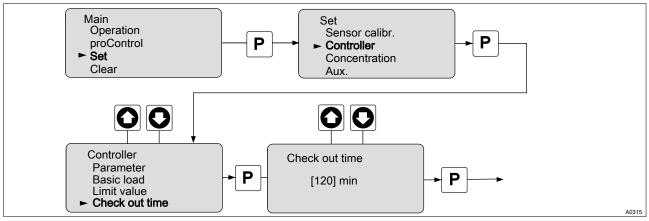
Fig. 19: Checkout time adjustment
