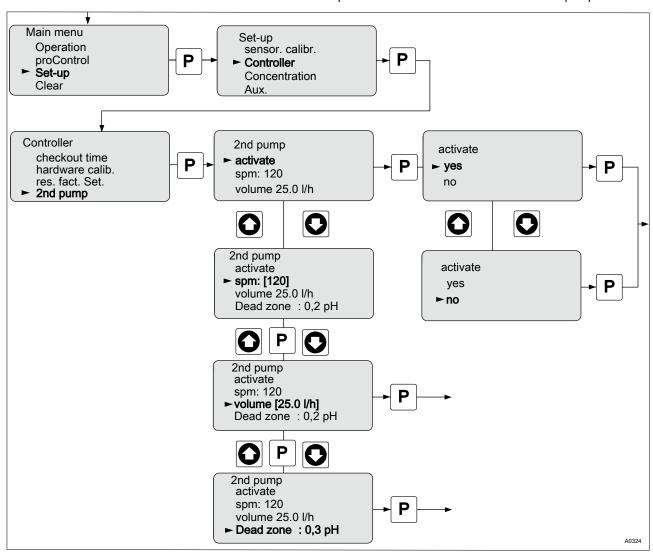
Fig. 22: Setting up "Two pump operation"
