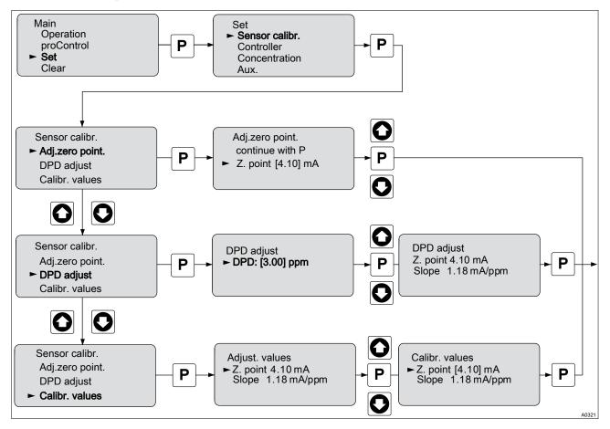
Fig. 26: Calibrating the sensor for chlorine
