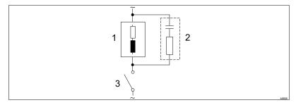
Fig. 10: RC protective circuit for the relay contacts
