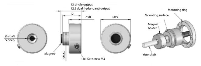
Note: If your shaft is magnetic, a minimum distance of > 1mm must be maintained from end of shaft to magnet.
