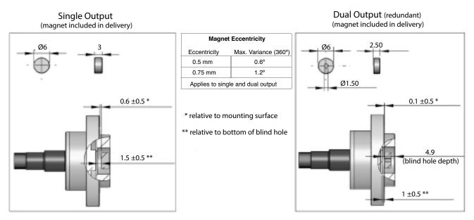
Note: If your shaft is magnetic, a minimum distance of > 1mm must be maintained from end of shaft to magnet.
