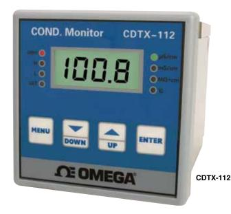
Resolution: 0.01 MΩ CDTX-111: 0.01 to 1 µS/cm CDTX-112: 0.01 to 0.01 mS/cm Temperature: 0.1°C (32.1°F) Accuracy: ±1% FS, ± 0.2°C **Temperature:** Automatic/manual Compensation: 0 to 100°C (32 to 212°F) Output Relays: 2 programmable, 10 A Control Type: On/off Relay Set Point Hysteresis: User programmable Current Output Type: Isolated 4 to 20 mA Range: Selectable zero and span Accuracy: ±0.02 mA Maximum Load: 750  $\Omega$ Power Supply: AC 110V to 220V ±10%, 50/60 Hz
