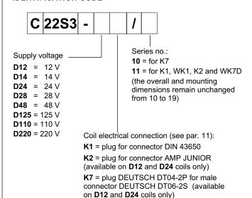
For W7 version only (D12 and D24 only) WK1 = plug for connector DIN 43650 WK7D = plug DEUTSCH DT04-2P, for male connector type DEUTSCH DT06-2S.
