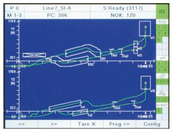
Figure: Display showing the two measurement curves  $Y_{+}(X)$  and  $Y_{-}(X)$
