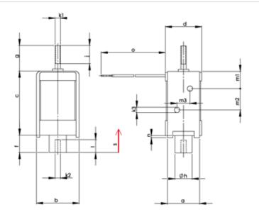
Armature position shown in currentless condition
