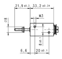
Armature position shown in energised condition
