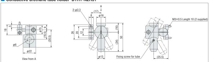
Note: For use with **DTRY-ADN-U** conductive urethane tube only. Cannot be used with **DTRY-ADN-F** Teflon tube or **DTRY-ADN-S** silicon tube.
