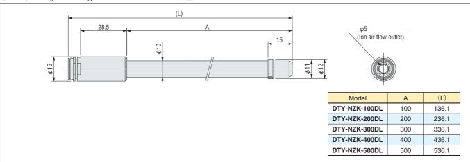
■ Low particle generation type straight bar nozzle DTY-NZK- □ 00BL
