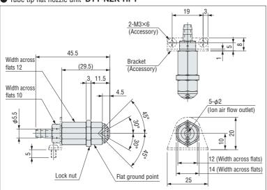
■ Tube tip bar nozzle unit DTY-NZK-H □ 00B
