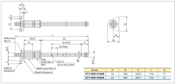
Remarks 1: Loosen the nut when adjusting the ionized air flow outlet direction. The recommended tightening torque for nuts is 70 to 90 N-cm.
