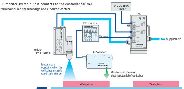
Static charge removal and particle removal using intermittent ionized air blowing
