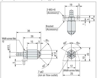
Tube tip flat nozzle unit DTY-NZK-HFT
