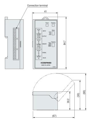
• Controller unit (solenoid valve built-in) **DTY-ZKCRU**
