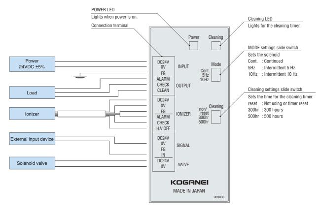
Note: Always be sure to connect the IONIZER H.V OFF terminal.
