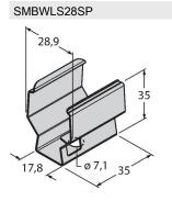
Snap bracket for mounting WLS28 work lights
