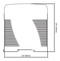
Figure 4 - Side view of Power Supply unit
