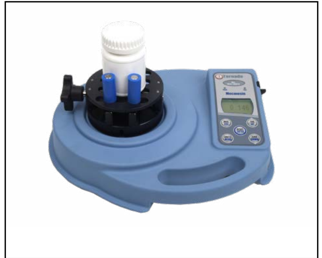
Small Saddle Plate (432-407) shown fitted to the small Lower Fixing Plate of the Tornado 1.5 N.m
