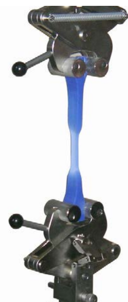
Mec11-20 with Mec11-20-BPR jaws shown testing dumbbell specimen
