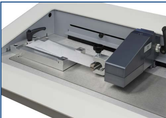
180° peel of self-adhesive labels (with part no. 432-636) ▲
