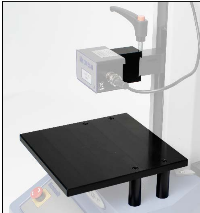
▲ Crosshead Extension and Elevated Base Plate
