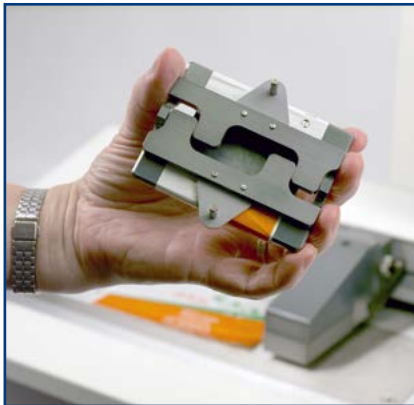
▲ 432-638: 200 g foam faced: ASTM D1894, ISO 8295
