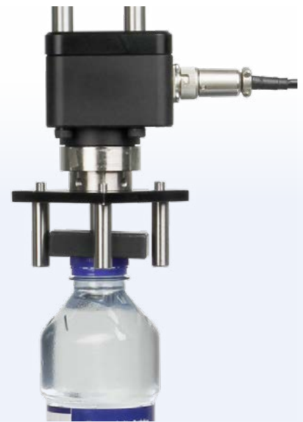
▲ Dedicated mandrel with drive holder to test TE bridge torque
