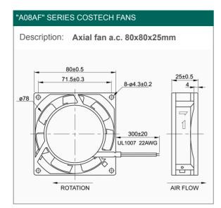
Casing material: aluminium die casting alloy ADC-12 black fibreglass reinforced plastic (PBT) UL Impeller material
