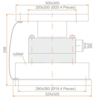
Maintains a stable measurement in weighing systems where vibrations and impact loads are present
