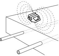
Estimating line depth using the C.A.T4+/eC.A.T4+ and Genny4
