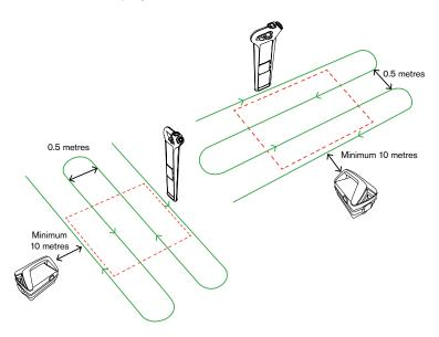
Active search using Induction – finding parallel pipes and cables
