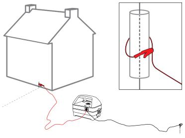
Signal jumping from an accessible cable
