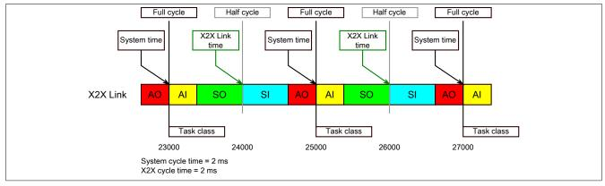
The reference time on the X2X Link network is always formed at the half cycle of the X2X Link cycle. This results in a difference between the system time and the X2X Link reference time when the reference time is read out.
