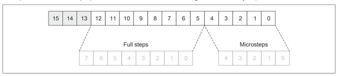
The number of transfer values per X2X Link cycle is specified by bits 3 and 4 in the module configuration (see "Module configuration" on page 20). If only one transfer value (bits 3 and 4 = 00) is specified, then the motor is advanced by MotorXStepX until the next X2X Link cycle. If 2 or 4 transfer values are specified, then the X2X Link is subdivided accordingly.
