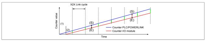
At startup, the internal counters for the PLC/POWERLINK (1) and the I/O module (2) start at different times and increase the values at µs intervals.
