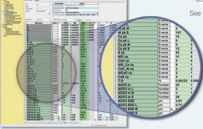
Detail of OXSAS display showing the result of simultaneous elemental concentration and inclusion analysis of a low alloy steel sample. The top results in % are from elemental analysis. All other results are from Spark-DAT methods. They include Al sol, Al insol and total oxygen (TO), peaks and coincidental peaks, and inclusion size.
