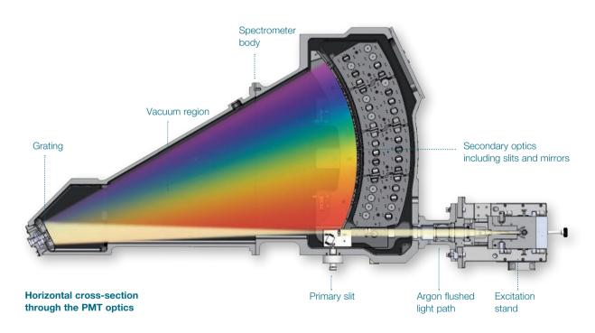
The spectrometer body is made of cast iron, operates under clean vacuum and is temperature controlled for ultimate stability, simplifying operation for users. PMT's with the most advanced signal acquisition and processing technologies offer the best possible performance available on the market. These attributes yield unmatched performances on all major, minor, and trace element constituents over short and long-term periods.
