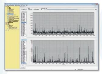
Single Spark Analysis charts allowing visualization of the inclusion signals of the two elements Al and Ca in steel
