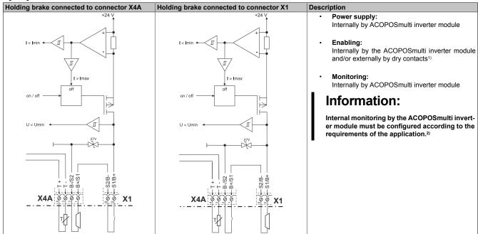
Table 16: Activation of the motor holding brake internally and/or externally
