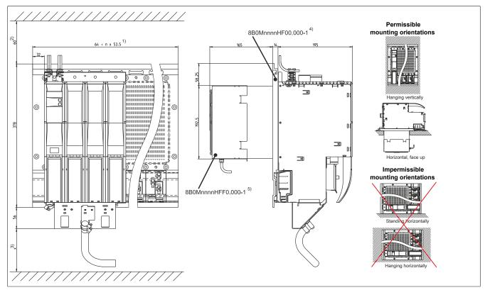
Figure 5: Pass-through mounting - Dimension diagram and installation dimensions
