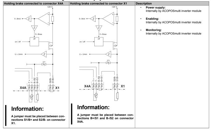
Table 15: Activation of the motor holding brake internally
