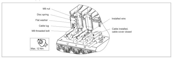
Figure 7: Motor connections U, V, W - Cable installation
