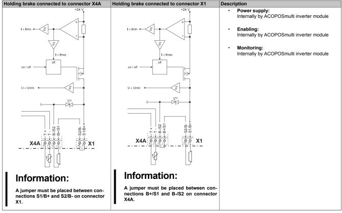
Table 10: Activation of the motor holding brake internally
