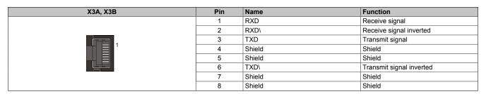
Table 13: X3A, X3B connectors - Pinout
