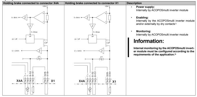
Table 11: Activation of the motor holding brake internally and/or externally
