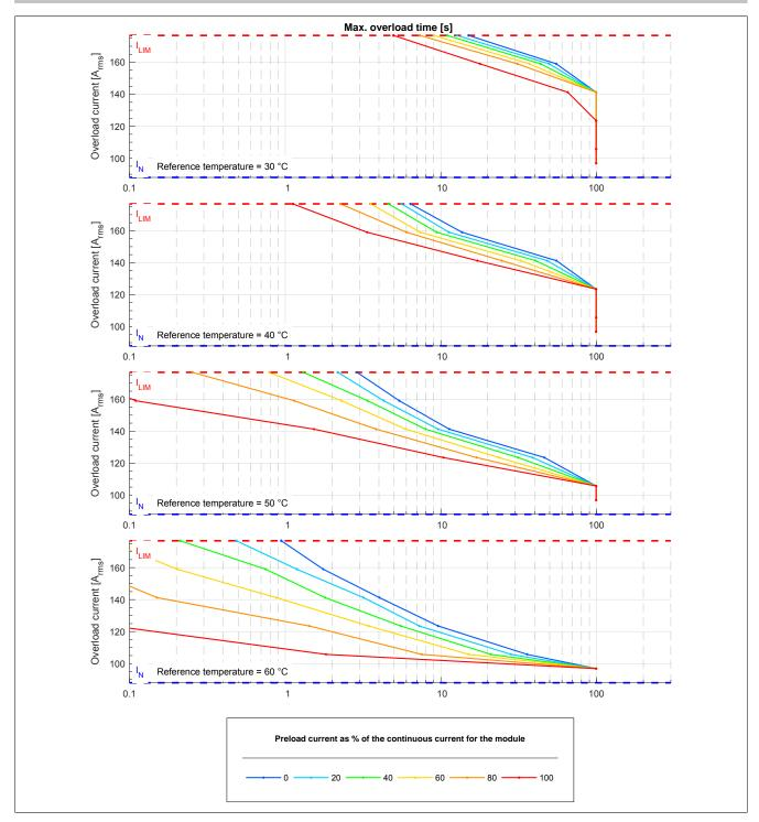
Figure 1: 8BVI0880HCSx.008-1 - Overload characteristics, overload response - WARNING
