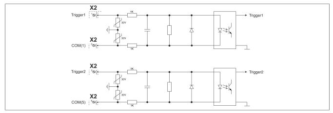
Figure 9: Trigger inputs
