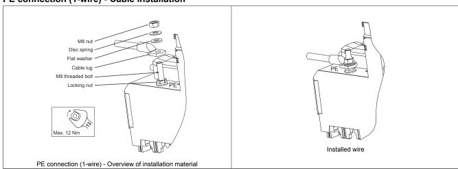
Table 18: PE connection (1-wire) - Cable installation
