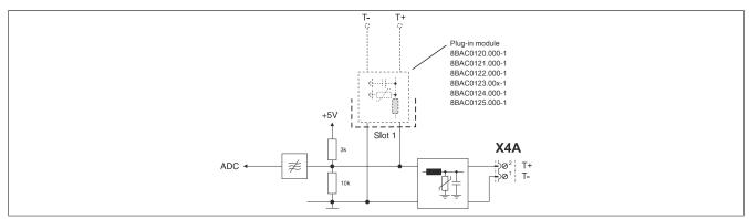
Figure 12: Temperature sensor
