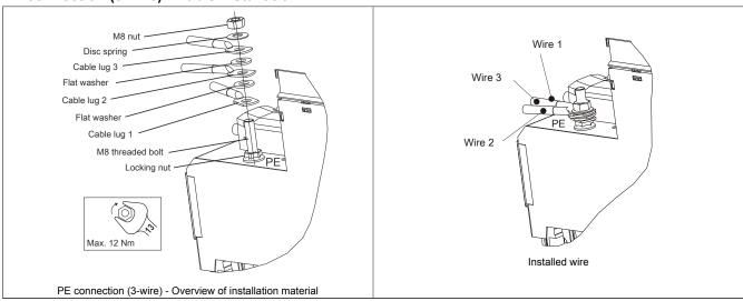
Table 19: PE connection (3-wire) - Cable installation
